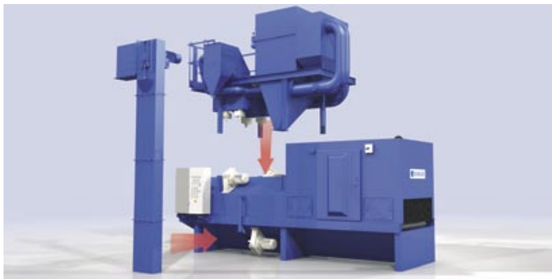
Automatic blasting of various semi-finished parts in continuous flow.
